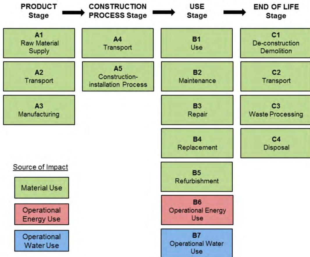
Figure 2: Stages contributing to the embodied carbon impacts over the life cycle of a building (Source: EN 15978:2011)
