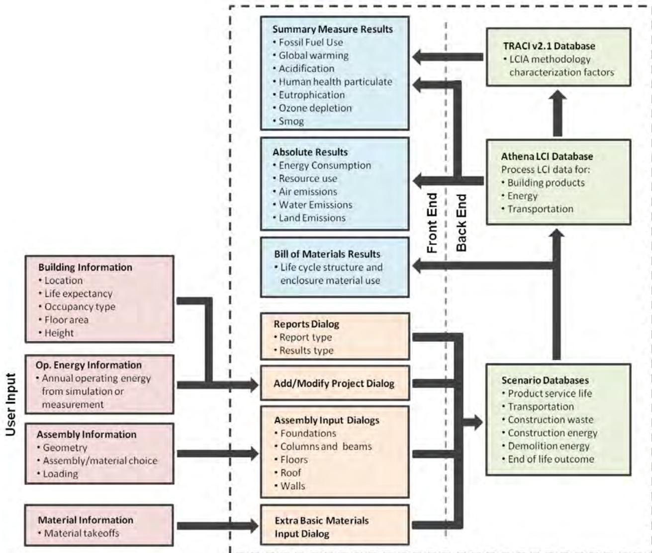
Figure 5: LCA Tool Sample Process from Athena IE4B (Source: Athena 2014)
