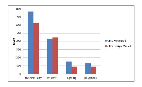
Figure 4: CIRS Annual Measured Energy Data versus Design Model Data
