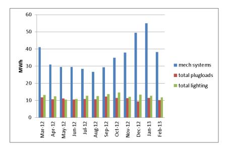
Figure 2: CIRS Monthly Measured Data Breakdown
